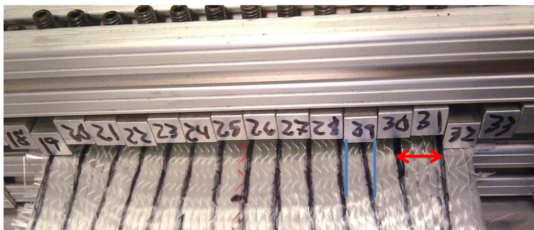
Figure 21. The tow misalignment after the initial displacement that can be seen in the fourth tow group (blue lines). It was caused by the cinching of the interior tow groups. The red arrow shows the second tow group stretched out to compensate.
