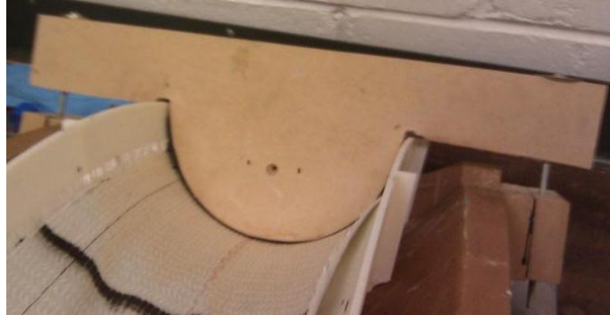
Figure 22. The pre-sheared fiberglass ply is placed into the mold and clamped at the seed position.
